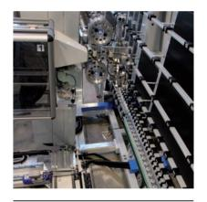
The flexible spacer is supplied by the manufacturer in a continuous role of approximately 500 meters wound directly onto a specifically designed bobbin. Product waste is kept to a minimum as is the downtime due to the quick and efficient system for changing from one bobbin to another.
